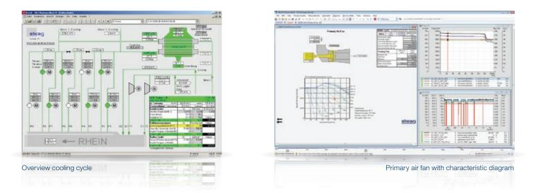
SR::EPOS is based on the thermodynamic cycle calculation program EBSILON<sup>®</sup> *Professional*. This calculation kernel allows to precisely assess the current plant condition by comparing results of a process simulation on the basis of inservice measurements with those of an EBSILON reference model in short intervals.
